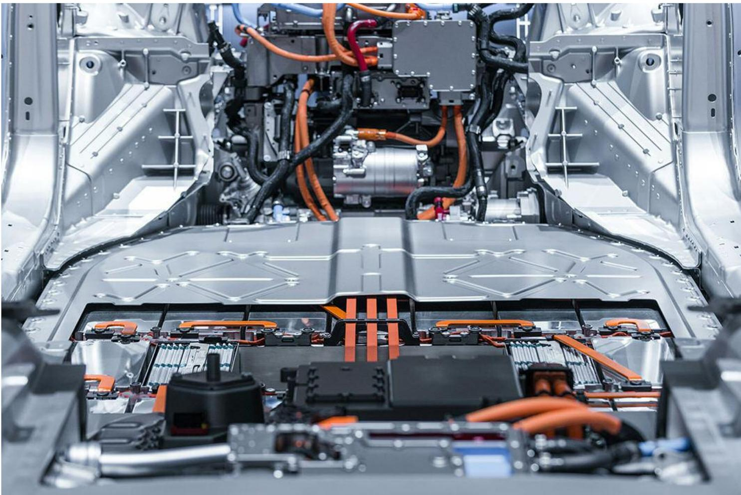
EVs bring a new requirement for coolant to be circulated around the vehicle and, more specifically, the battery
